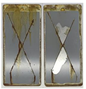
**Subject:** Plate 1 for MS 775 silica anti-corrosion pigments.
